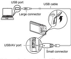
Making sure that the ◀ mark on the USB cable connector is towards the monitor screen side, connect the cable to the camera.
